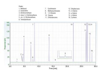
Figure 4. Comparison between Class 2A standard solution (blue) and acetylsalicylic solution (green). Criteria are met as no residual solvent peaks could be detected in the test sample.
