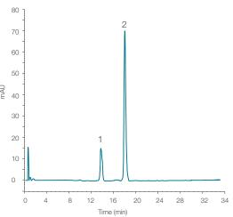
Figure 2. Improved analysis of ibuprofen and valerophenone using a Accucore C18 column
