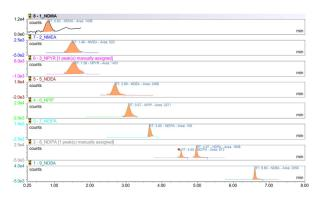
Figure 1. XIC of quantitation ion of nitrosamine impurities in 0.5 ng/mL check standard at a mass tolerance setting of 3 ppm
